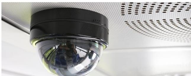
The video surveillance system begins recording every time a bus is started. Data and images are stored in the secure on-board Digital Video Recorder (DVR) hard drive.
