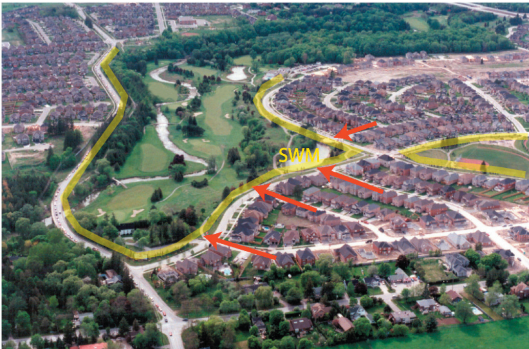
Photos 4 and 5: New development patterns are aligned to create open space connections to woodlots, hedgerows, stormwater ponds, and other natural features.
