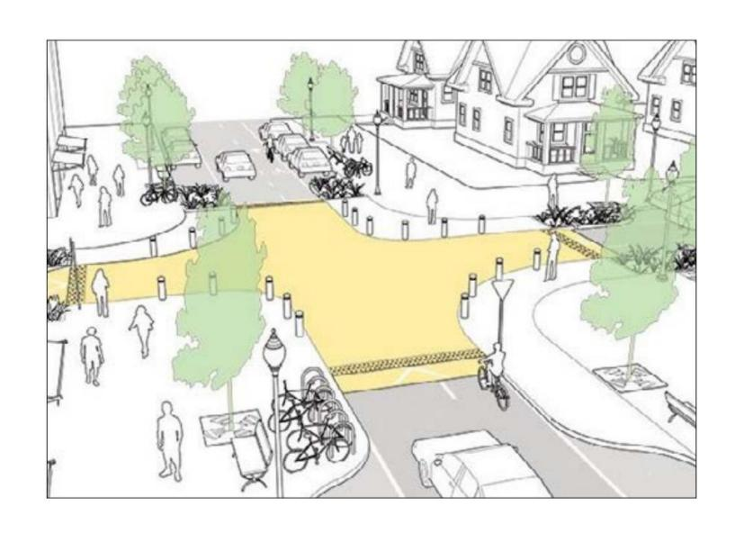
An intersection at a higher level than the roadway to discourage speeding and delineate the pedestrian crossing area
