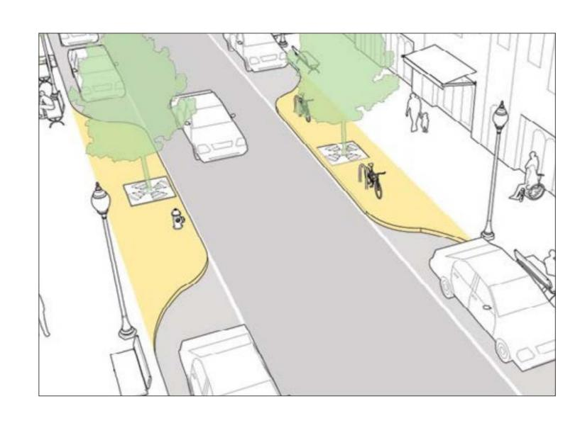
Provide a narrowing effect to reduce crossing distances and vehicular travel speeds through physical extensions of the curb and sidewalk
